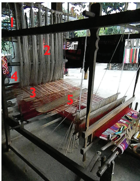
Figure 4. Six Khau components
